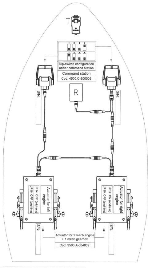
The actuator marked on the drawing identifies its position on the boat
