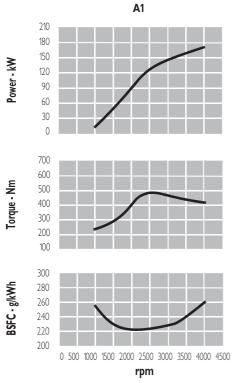
A1 = High performance crafts. Full throttle operation restricted within 10% of total use period. Cruising speed at engine rpm < 90% of rated speed setting - Maximum useage 300 hours per year.
