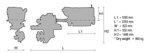
\*L= Length with supported elastic joint Vulkardan E and 370mm cardan shaft \*\*Dry weight without elastic joint - cardan shaft - propellers Publication P3D06N012E - 09.12 Specifications subject to change without notice. Illustrations may include optional equipment.
