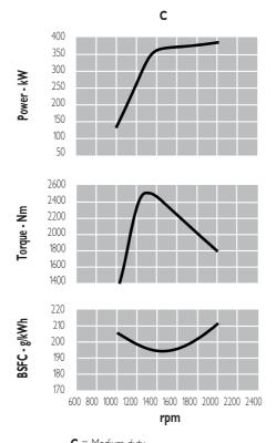
$\mathbf{C}$  = Medium duty. Full throttle operation < 25% of use period. Cruising speed at engine rpm < 90% of rated speed setting - Maximum useage 3000 hours per year.
